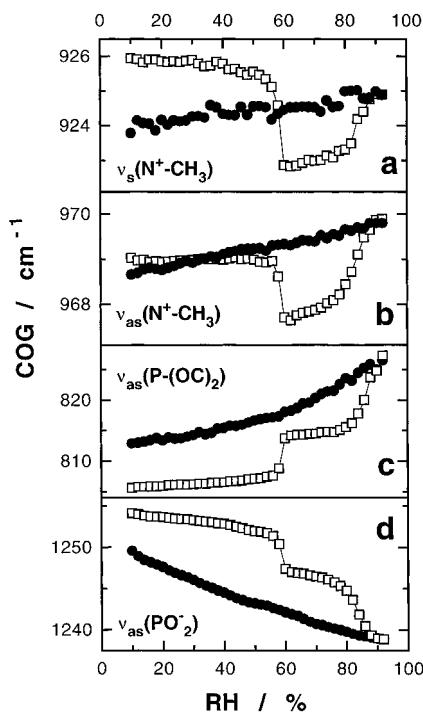
**Figure 8.** Center of gravity (COG) of absorption bands of the choline and phosphate groups of DODPC as a function of relative humidity (RH) obtained from hydration (□) and dehydration (●) scans: (a)  $\nu_s(N^+-CH_3)$ ; (b)  $\nu_{as}(N^+-CH_3)$ ; (c)  $\nu_{as}(P-(OC)_2)$ ; (d)  $\nu_{as}(PO_2^-)$ .
