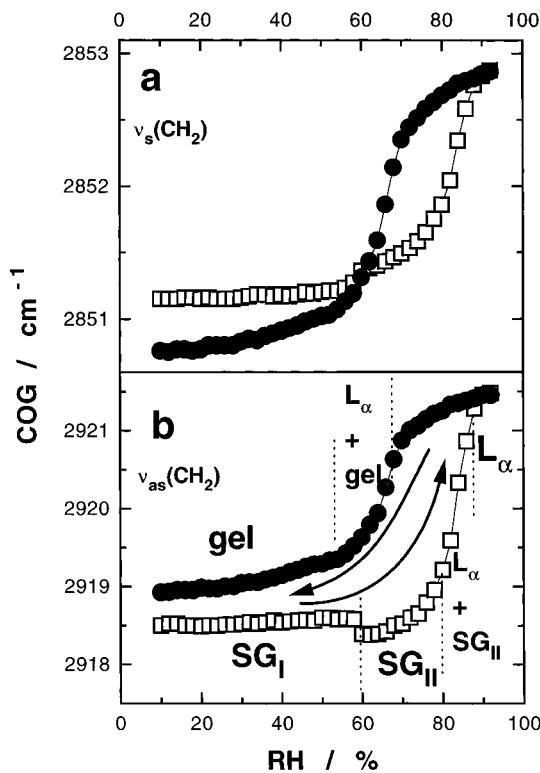
**Figure 1.** Center of gravity (COG) of the symmetric (a) and antisymmetric (b) CH<sub>2</sub> stretching bands,  $\nu_s(CH_2)$  and  $\nu_{as}(CH_2)$ , of DODPC as a function of relative humidity (RH) obtained from hydration (□) and dehydration (●) scans. The corresponding phase sequences are indicated in part b.
