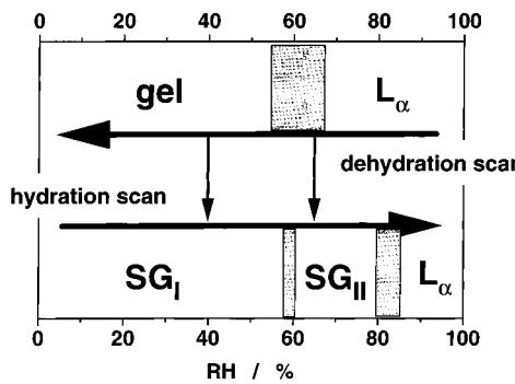
**Figure 4.** Schematic illustration of the phase sequences passed upon gradual dehydration and hydration of DODPC. Phase coexistence regions are shown by gray areas. The smaller arrows indicate transitions to the subgels.
