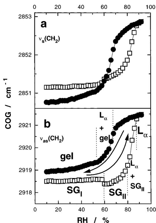
**Figure 1.** Center of gravity (COG) of the symmetric (a) and antisymmetric (b)  $\text{CH}_2$  stretching bands,  $\nu_s(\text{CH}_2)$  and  $\nu_{as}(\text{CH}_2)$ , of DODPC as a function of relative humidity (RH) obtained from hydration ( $\square$ ) and dehydration ( $\bullet$ ) scans. The corresponding phase sequences are indicated in part b.
