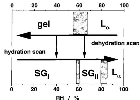
**Figure 4.** Schematic illustration of the phase sequences passed upon gradual dehydration and hydration of DODPC. Phase coexistence regions are shown by gray areas. The smaller arrows indicate transitions to the subgels.
