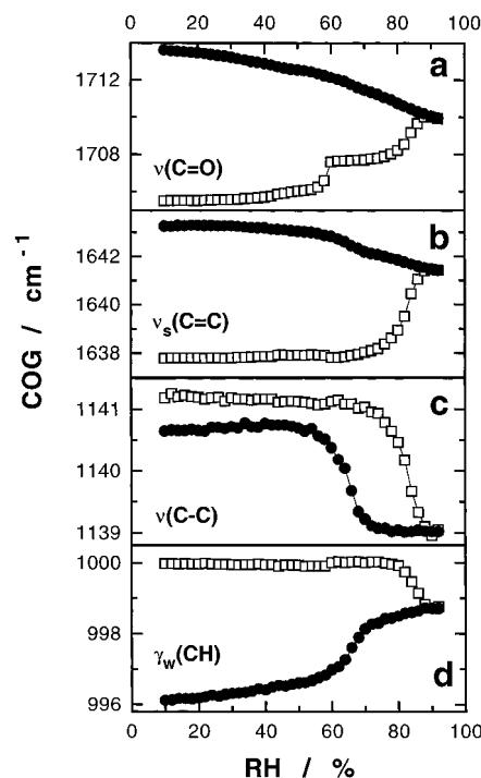
**Figure 9.** Center of gravity (COG) of absorption bands of the carbonyl and diene groups of DODPC as a function of relative humidity (RH) obtained from hydration (□) and dehydration (●) scans: (a)  $\nu(C=O)$ ; (b)  $\nu_s(C=C)$ ; (c)  $\nu(C-C)$ ; (d)  $\gamma_w(CH)$ .
