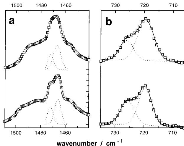
**Figure 5.** Absorbance spectra in the region of the CH<sub>2</sub> bending (a) and rocking (b) modes of DODPC in the SG<sub>I</sub> (bottom) and SG<sub>II</sub> (top) states. The conditions are the same as given in the legend of Figure 2. The Gaussian functions fitted to the bands are shown by dotted lines and their superposition by solid lines.
