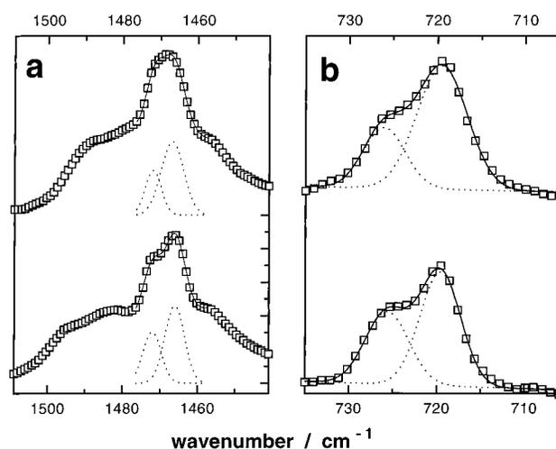
**Figure 5.** Absorbance spectra in the region of the CH<sub>2</sub> bending (a) and rocking (b) modes of DODPC in the SG<sub>I</sub> (bottom) and SG<sub>II</sub> (top) states. The conditions are the same as given in the legend of Figure 2. The Gaussian functions fitted to the bands are shown by dotted lines and their superposition by solid lines.
